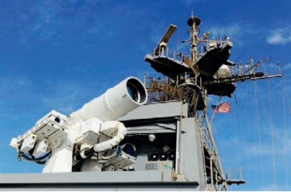
STANDING BY: The Laser Weapon System (LaWS), developed by the Office of Naval Research, undergoes testing on the USS Ponce in the Arabian Gulf in 2014. Futuristic devices such as high-energy lasers and microwave weapons promise a cost-effective way to counter unmanned systems and have drawn increased defense funding. Whether on ships, in the air, or on the ground, directed-energy weapons will need advanced sources of power. [John F. Williams—US Navy]
