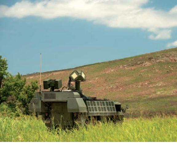
ON TARGET: A prototype Stryker armored vehicle takes the field in an Army exercise in Fort Sill, Oklahoma, last summer. The vehicle was testing lasers to defend against unmanned aircraft, rockets, artillery, and mortars. The directed-energy "shoot off" was declared a success and a "gateway to the future." [US Army]
