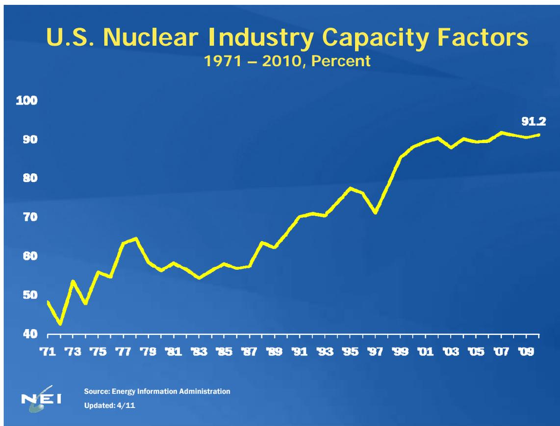
**Figure 1: United States Fleet-Level Nuclear Capacity Factors**
